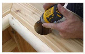
Screw the bar top to the side walls using a 2  $\frac{1}{2}$ " (64mm) screw by screwing on an angle through the post holes into the wall.
