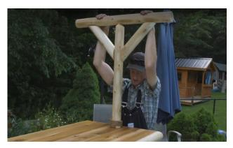
Slide the log T posts into each of the holes in the bar top.
