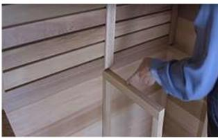
Align the middle support brackets to the supports on the bottom of the bench.
