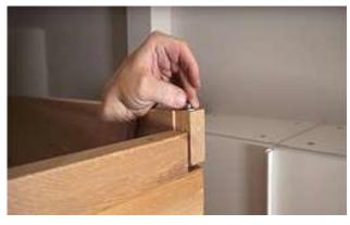
Place the washer then the nut on the threaded rods and tighten with the wrench.
