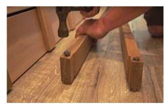
Tap the Provided (4) – "T-Nuts" into the holes on the bottom of the 2 side with a hammer.
