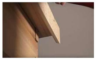
Using the rubber mallet, tap the roof trim into position.
