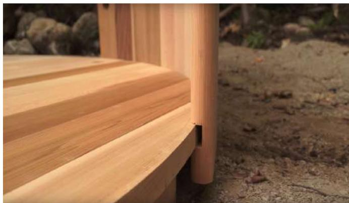
Leave a space between the edge of the floor and the bottom of the dado. Use the pencil line circle on the floor as a guide.
