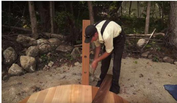
Start placing the staves with the dado (groove) over the edge of the floor as shown.
