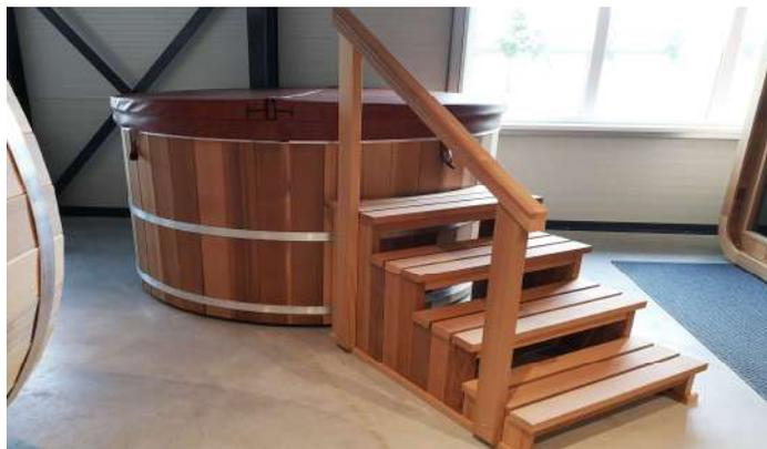
Place the assembled steps next to the tub and secure in place with two 2" screws through brackets under the top step.
