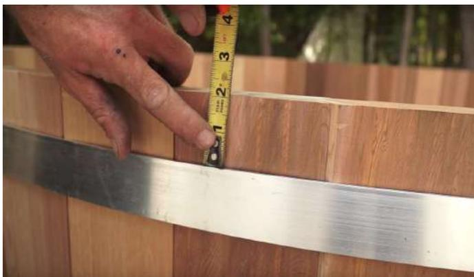
Using the same method as the bottom band, measure 2" from the edge of the top staves to the top of band.
