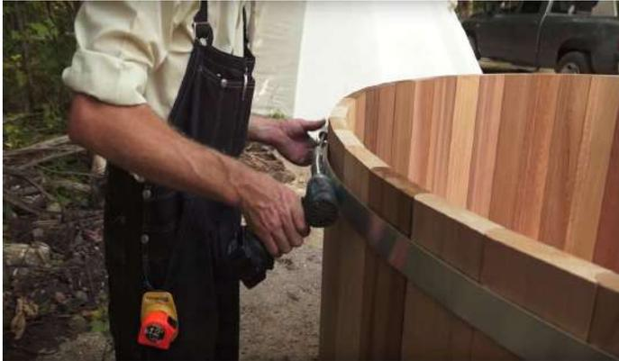
Tighten each band a little at a time, starting with the bottom band.
