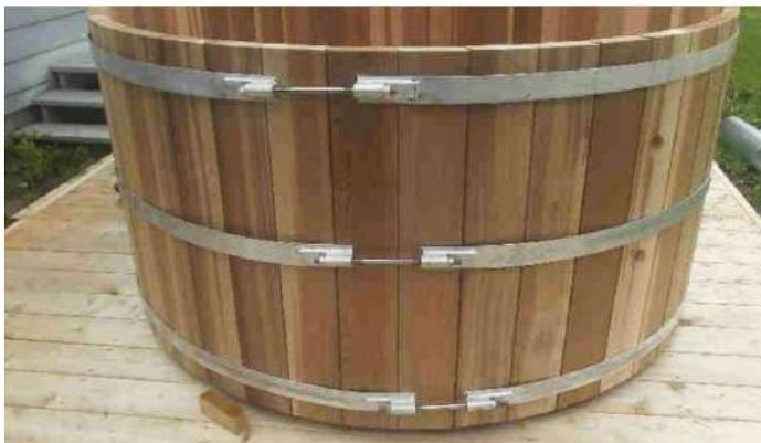
Assemble the other bands, and slip them into place with their tightening hardware rotated so that it is offset from the one below as shown.
