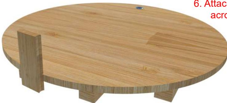
7. Continue to add the short bottom staves using a rubber mallet if needed to ensure they are tight.
