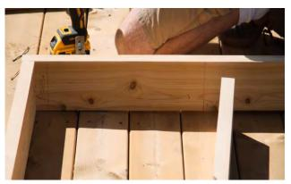
The front and back pieces will be "marked" where each of the base supports will be placed.
