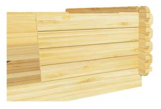
Install the medium length stave labelled "window" on either side of the front wall and secure in the same manner as previous steps.
