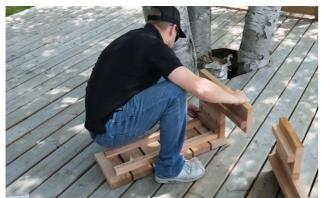
To assemble the 2-tier step (if ordered), place the top step upside down and a stair support on top.
