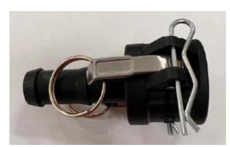
Connect the cam lock of the completed tubing line to the "Inlet" of the chiller.
