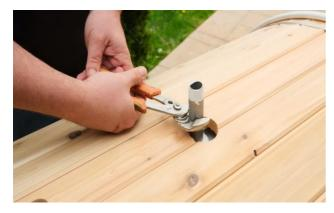
Thread one of the long pieces of pipe into the top hole on the side of the tub tightening with a pipe wrench.
