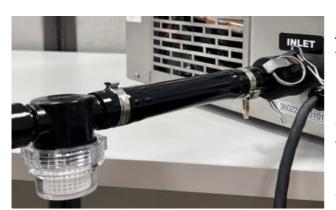
Attach the in-line strainer to the other end of the 6" tubing.
