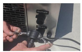
Attach the cam lock to the "outlet" of the chiller.
