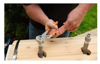
Thread a quick connect onto each of the long pipes.
