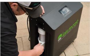
Insert the filter into the holder and screw onto the chiller. Tighten with the provided filter tool.
