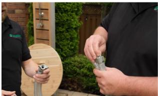
Insert rubber washers into each end of the chiller hoses.
