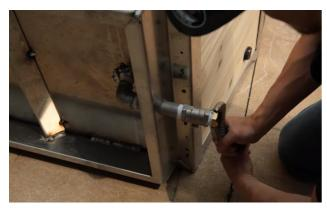
Using a pipe wrench or adjustable wrench, tighten the garden hose connector onto the valve.
