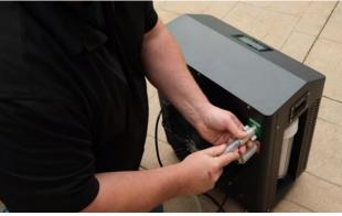
Screw the chiller hoses onto the inlet and outlet connections, Ensure they are tight.
