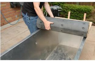
To open the cover, unclasp the straps and roll up the cover to sit on the cover supports.
