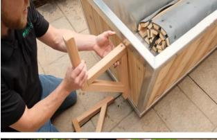
To install the roll up cover, secure the cover brackets onto the preferred end of the plunge tub and secure with  $2 - 2 \frac{1}{2}$ " (64mm) screws into each bracket.
