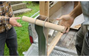
Slide the dowel through the hole in the rigger so it is even on both sides.
