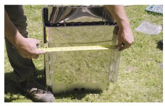
To start the installation of the electric heater, measure the width of the stove mounting holes.
