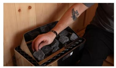
Carefully place the rocks loosely between the heating elements until the heater is filled.
