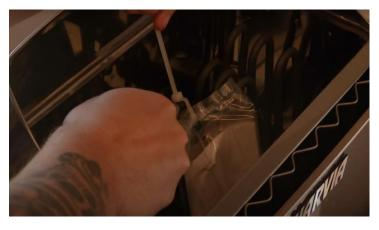
Cut the zip tie and remove the temperature sensor guard and put aside as it will be needed in future steps.
