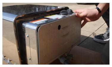
Replace the bottom panel ensuring the red "high limit" button is accessible through the designated hole, if not adjust the panel accordingly.
